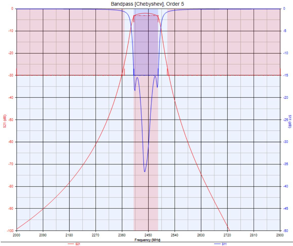
Figure 3 Simulated performance of optimized filter on RT/Duroid 5870 material
