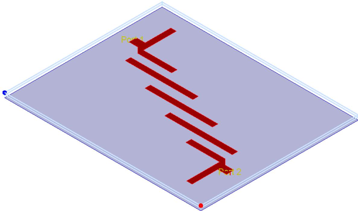
Figure 6 Physical appearance of RT/Duroid 5870 bandpass filter
