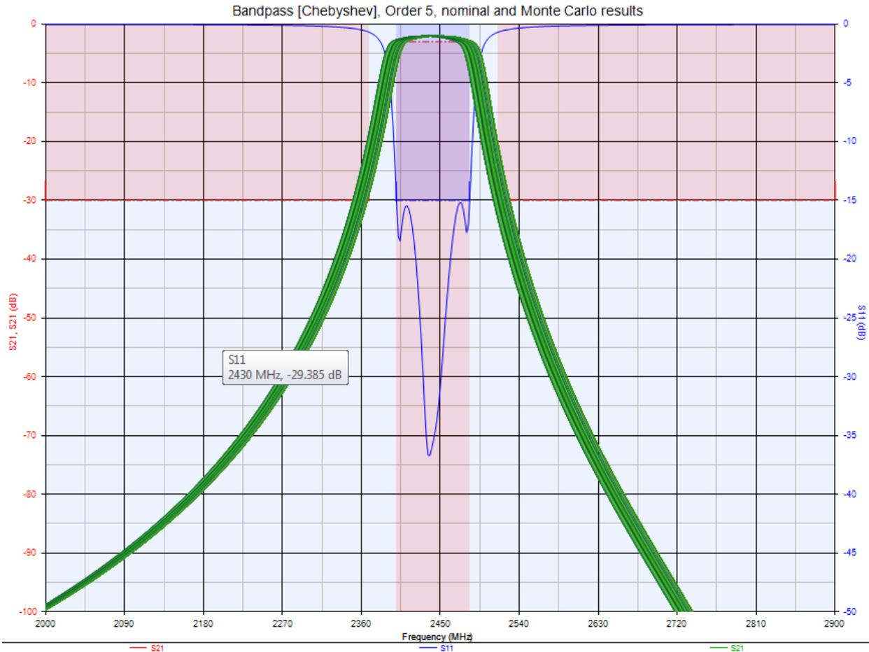
Figure 4 Monte Carlo analysis of RF/Duroid filter
