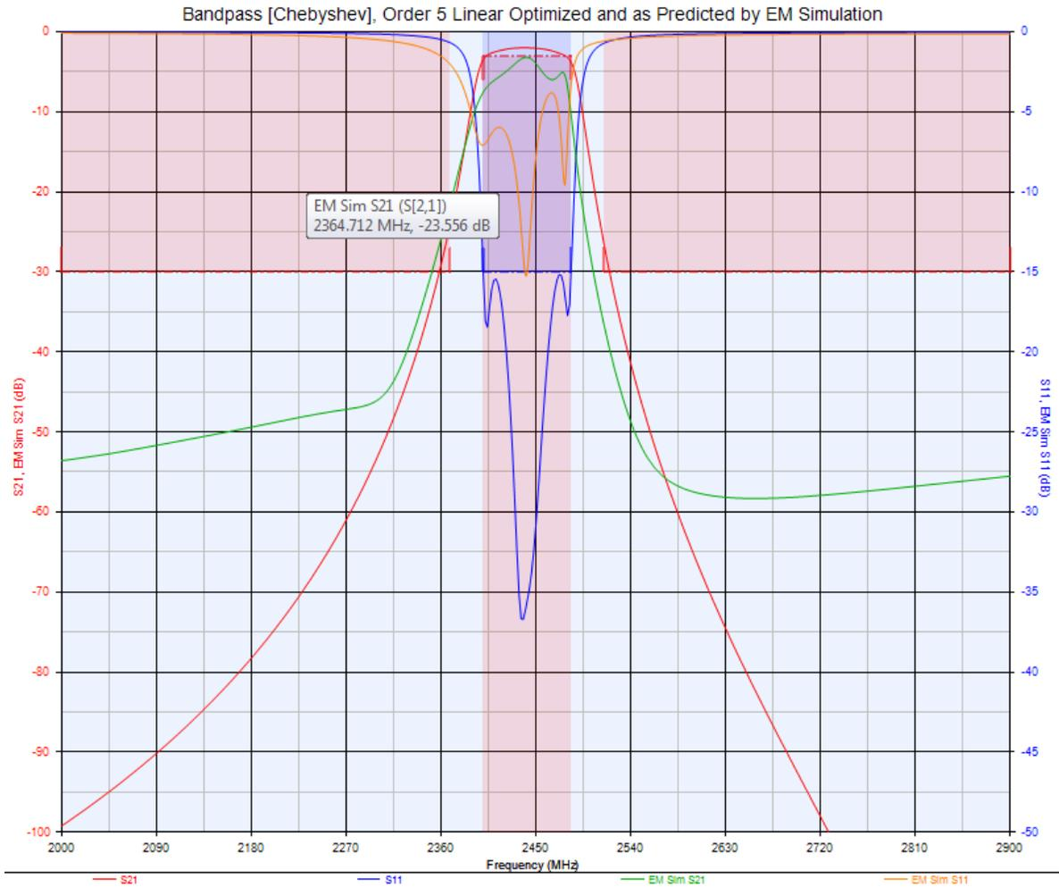
Figure 5 RT/Duroid 5870 linear and EM simulation predictions
